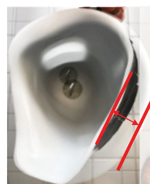
Figure 5. An overlay of images B and D in Figure 4 in the transverse view of the socket fully opened and fully tightened.
